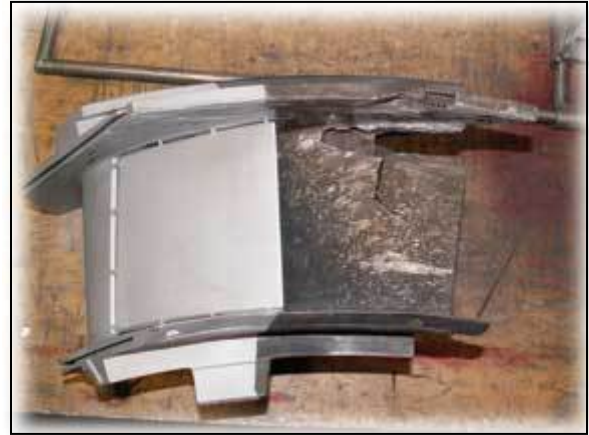
Even severely damaged nozzle blades can be cut out and a trailing edge coupon dropped into place ready for welding. Photo courtesy of Frarendi.
