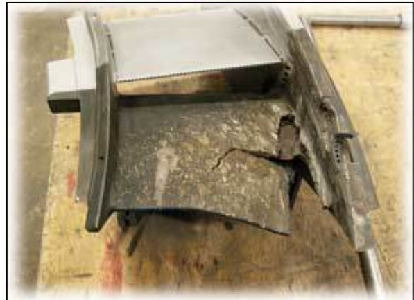
This Stage 1 nozzle segment has a coupon with trailing edge cooling holes as drilled with EDM process.
